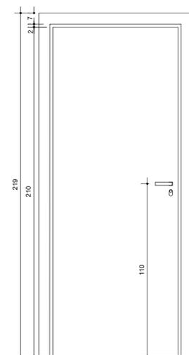
PORTA SIMPLES TIPO PRANCHETA, SEMI-OCA, PADRÃO MÉDIO, COM ESPESURA DE 3,5CM, COM MAÇANETA DO TIPO ALAVANCA COM CHAVE, ACABAMENTO PINTURA ESMALTE SINTÉTICO ACETINADO.
